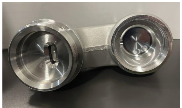
Finished forged aluminum shock body caps
